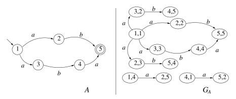
**Fig. 7.** An example of a state-pair graph  $G_A$  for a given finite-state automaton A. We omit all nodes that have no out-transitions in  $G_A$ .
