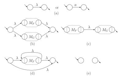
**Fig. 1.** The Thompson construction. Let E, F and G be regular expressions and  $M_F$  and  $M_G$  be the corresponding Thompson automata for F and G, respectively. (a)  $E = a + \lambda$ , (b) E = F + G, (c)  $E = F \cdot G$ , (d)  $E = F^*$  and (e)  $E = \emptyset$ .
